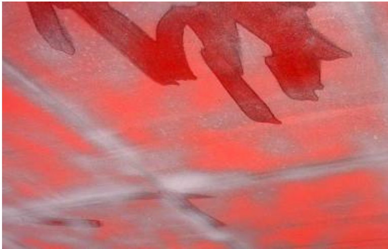
The dark area at the top of the photograph shows the extent of oil contamination after cleaning.
