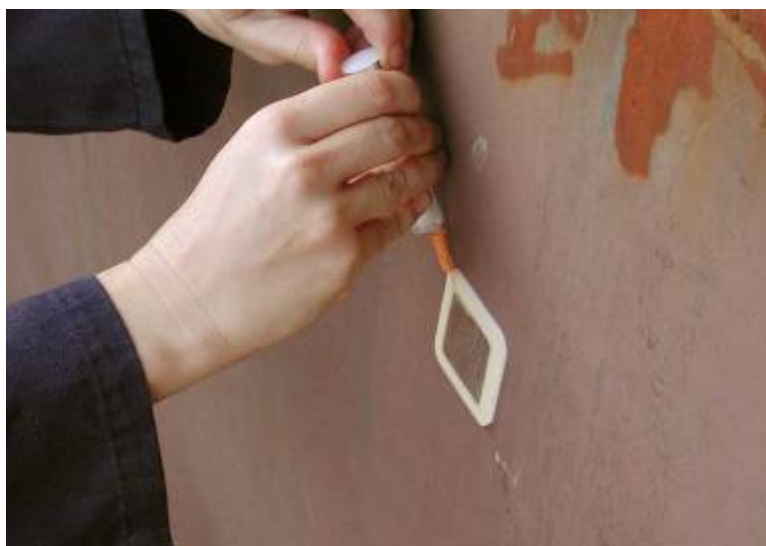
PHOTOGRAPH 1 Salt Contamination Testing
