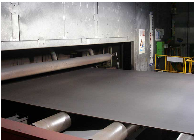
PHOTOGRAPH 10 Steel Plate after Blasting on the Shop Primer Line
