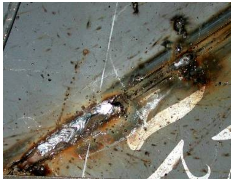
PHOTOGRAPH 9 Weld Fume (Brown Stains) and Spatter
