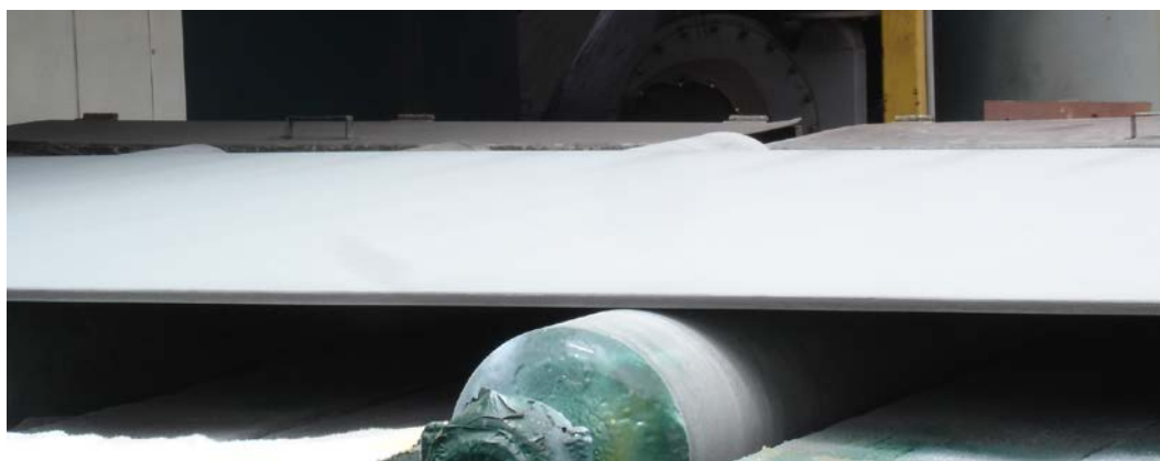
PHOTOGRAPH 12 Steel Plate Coated with Shop Primer (1 January 2017)
